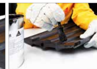
Applying the vulcanizing solution to the rubber surface
