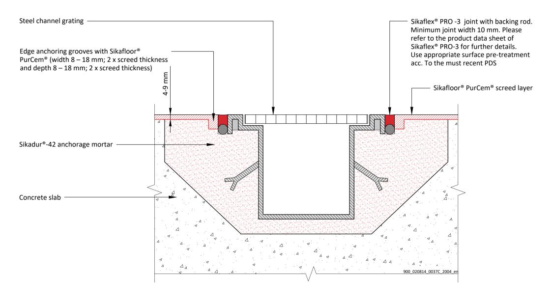
Sikafloor® PurCem® Drainage channel detail
