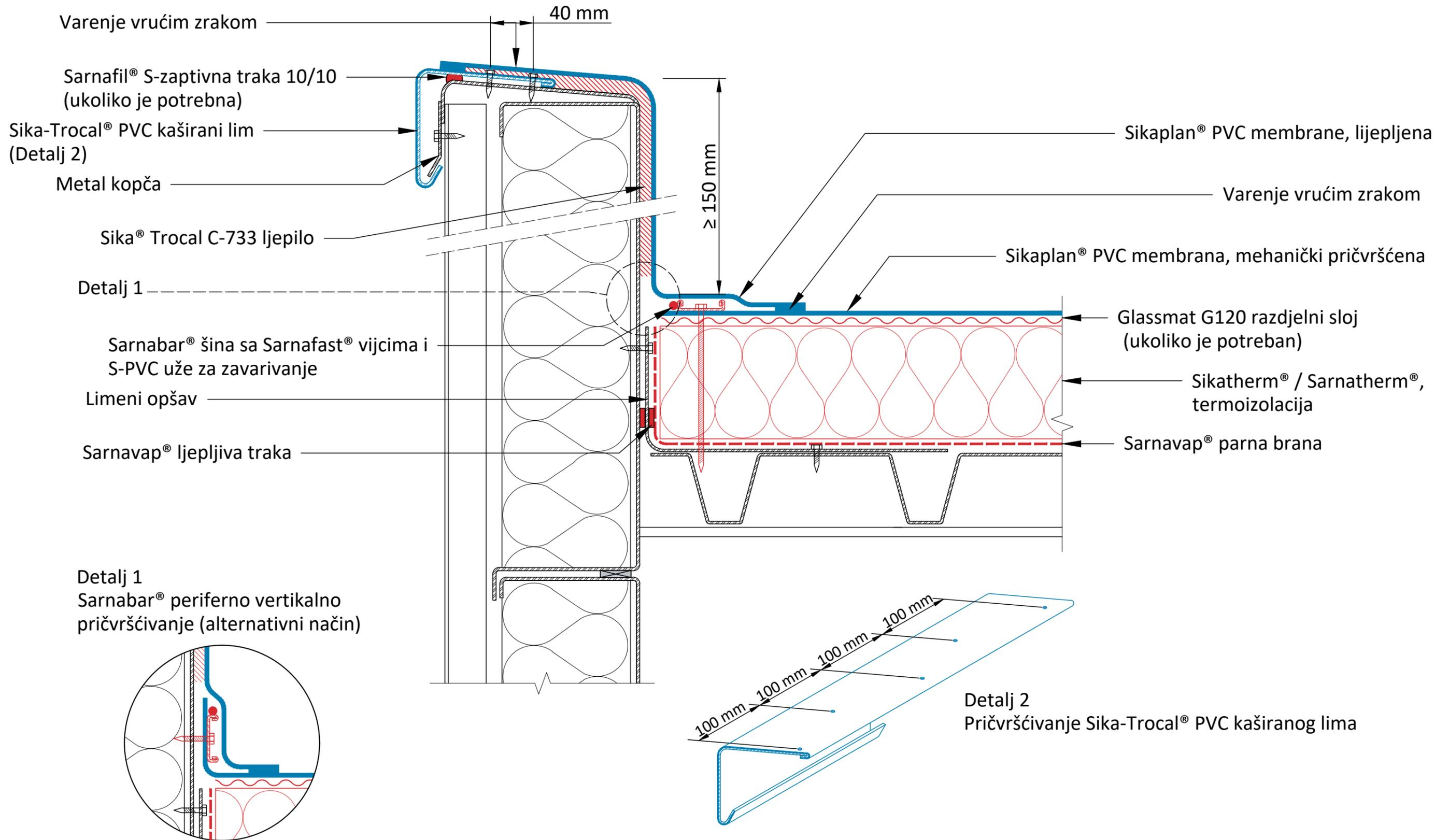
**SIKAPLAN® PVC - MEHANIČKI PRIČVRŠĆENI SISTEM
